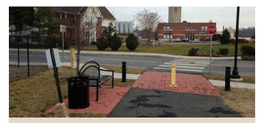
Figure 19—Multi-Use Trail Approach to Sidewalk Intersection & Mid-Block Crossing, Milton, DE
